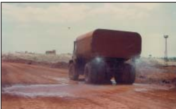
Water Sprinkler at Mine, NALCO
